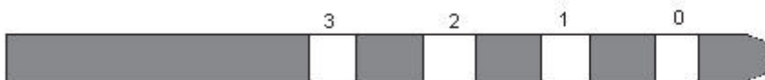
Figure 1. Quadripolar Pisces Quad lead with 4 contacts (0,1,2,3) at its distal end. The cylindrical contacts have a diameter of ~1.3 mm, are 3 mm long and are separated by 6 mm.
